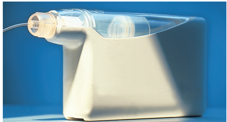
The 106 Microdialysis Pump is a small, lightweight, battery-powered syringe pump. It can be attached to the patient or placed on the bed. Its unique design makes operation simple, and the preset 0.3 \mu L/min flow results in high recovery of the substances from the extracellular fluid.
