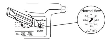
The normal flow can be adjusted in eight different flow rates by the switch at the back of the pump.
