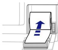
3. Replace the paper making sure that the free end of the paper comes out from the bottom of the paper roll
