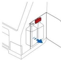
3. Replace the Rinse bottle (wide neck front bottle) with a new bottle of Rinsing Fluid (REF 8002171)
