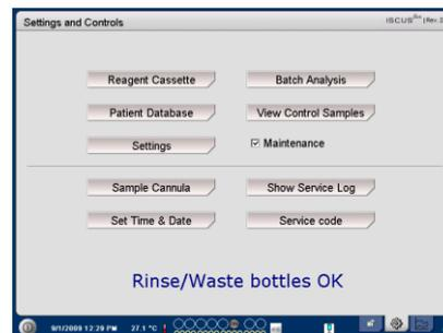
The Service Log shows calibration factors and solvent blanks. The Service Log also shows error messages and other important messages for Service engineers
