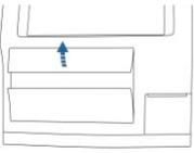
2. Lift up and remove the upper lid. This will expose the interior of ISCUS<sup>flex</sup> and makes it possible to locate the position of the sample cannula
