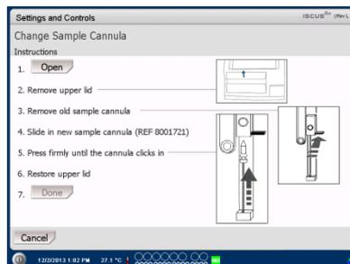
**NOTE!** Do not touch the tip of the cannula as it can cause needle injuries and be contaminated. Be sure to follow hospital infection risk procedures
