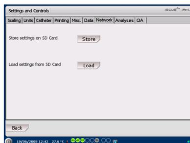
**NOTE!** If the load button is still shaded after a SD card/USB memory is inserted there are no settings on the device to load
