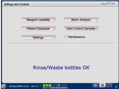
Check mark the Maintenance check box to gain access to additional functionality
