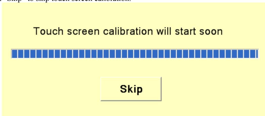
If you do not select “Skip”, the touch screen calibration sequence will start. Follow the instructions shown on the screen. When the calibration has ended, press on the center of the screen to end the calibration sequence.
